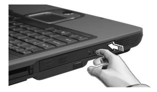
When the power is off, you can eject the drive tray using the emergency eject hole. See page 64.
